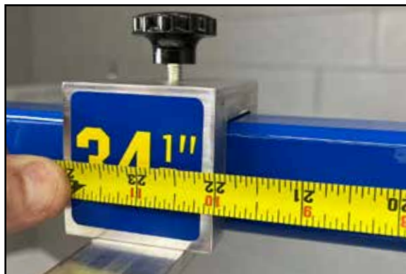
SET LEFT SIDE QUARTER HEIGHT BLOCK TO 22 INCHES FROM END OF REFEREE
