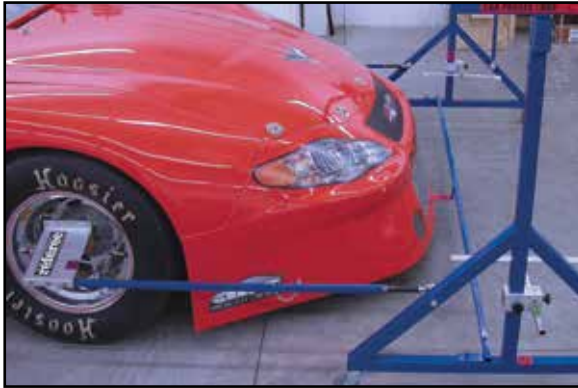
INSERT ARMS INTO FRONT WHEELS & LOCK INTO PLACE.
