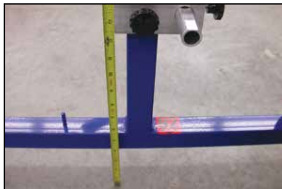
ADJUST BLOCK SO TREAD WIDTH GAUGE IS LOCATED TO CENTER OF WHEEL (APPROXIMATELY 12-½ INCHES UP FROM GROUND). THIS DIMENSION WILL VARY BASED ON TIRE SIZE.
