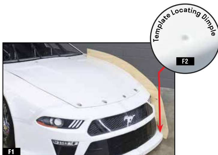
LEFT SIDE TEMPLATE IS LOCATED 21-3/4 INCHES FROM CENTERLINE.
