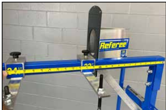
BEGIN BY MEASURING FROM THE END OF THE REFEREE TO LEFT QUARTER HEIGHT BLOCK
