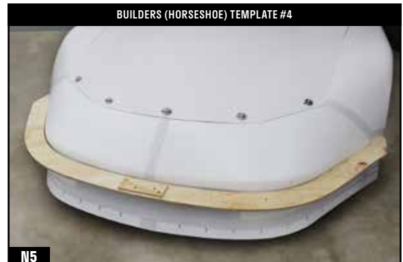
THIS TEMPLATE SHOULD BE PLACED APPROXIMATELY 1-1¼" ABOVE THE TOP OF THE NOSE SCREEN, AND PARALLEL TO THE GROUND.
