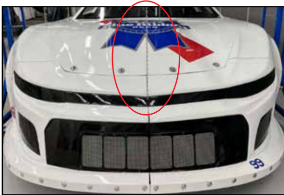
THE BODY CENTERLINE CHAIN SHOULD BE ON CENTERLINE OF THE NOSE +/- 1" TOLERANCE FOR VARIABLES SUCH AS CAMBER, TREAD WIDTH, AND OTHER CONTRIBUTING FACTORS
