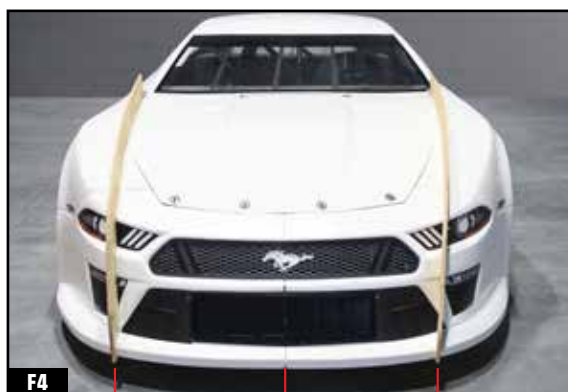
BOTH FENDER TEMPLATES ARE LOCATED AT THE INTERSECTION OF THE FENDER AND HOOD AT THE REAR OF THE TEMPLATE.
