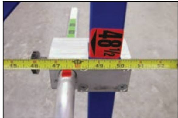
ADJUST HEIM ON FORWARD ARM TO OBTAIN 48- \frac{1}{2} INCH MEASUREMENT. REPEAT PROCESS FOR OPPOSITE ARM.
