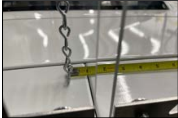
NEXTGEN BODY REAR CENTERLINE OF BUMPER COVER IS 1 INCH TO THE RIGHT TRADITIONAL BODY REAR CENTERLINE IS ON THE BUMPER COVER CENTERLINE
