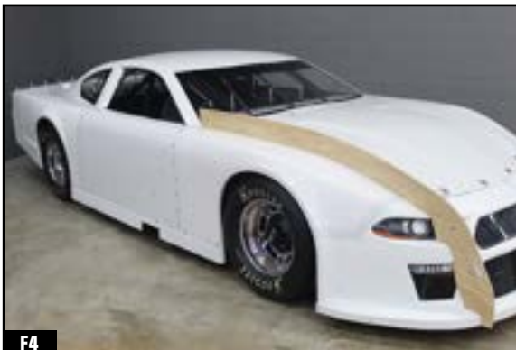
RIGHT SIDE TEMPLATE IS LOCATED 24-3/4 INCHES FROM CENTERLINE.
