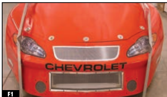
LEFT SIDE TEMPLATE IS LOCATED 23-7/8 INCHES FROM CENTERLINE. RIGHT SIDE TEMPLATE IS LOCATED 26 INCHES FROM CENTERLINE.
