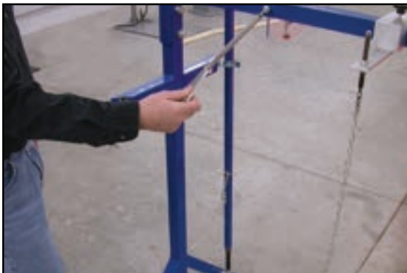
ADJUST HEX ROD TO OBTAIN 92 INCHES FROM OUTSIDE TO OUTSIDE OF DEVICE.
