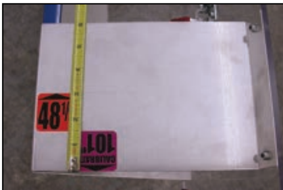
LEAVE FORWARD ARM (THAT WAS JUST CALIBRATED) IN THE HORIZONTAL POSITION ON THE 13- \frac{1}{4} INCH BLOCKS. PLACE REARWARD ARMS IN HORIZONTAL POSITION ON ANOTHER 13- \frac{1}{4} INCH BLOCK. HOOK TAPE MEASURE ONTO FORWARD ARM ON THE 101 INCH STICKER & EXTEND TAPE TO REARWARD ARM AT 101 INCH STICKER.
