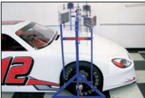
INSERT LEFT SIDE THREAD WIDTH MEASURING ARM INTO LEFT WHEEL & LOCK INTO PLACE. REPEAT THIS PROCEDURE ON THE RIGHT SIDE.
