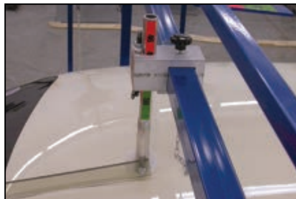
THE ROOF HEIGHT IS MEASURED BY VIEWING THE CALIBRATED ROD ATTACHED TO THE POLYCARBONATE GAUGE.
