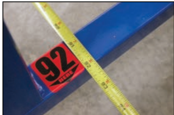
THE 92 INCH DIMENSION IS CRITICAL TO ENSURE TREAD WIDTH GAUGES ARE PROPERLY CALIBRATED.
