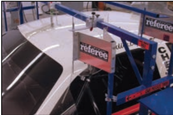
MOVE CAR OR REFEREE UNTIL ROLLER CONTACTS ROOF & POLYCARBONATE GAUGE IS IN LINE WITH THE TOP EDGE OF THE WINDSHIELD
