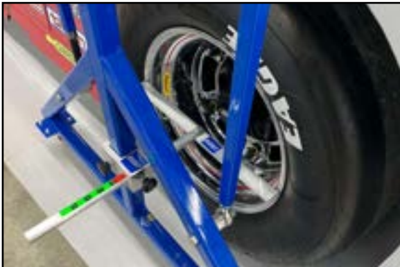
LOCK THE RIGHT FRONT AT 66 INCHES
