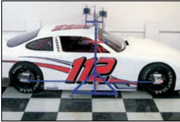
INSERT FRONT ARM INTO THE FRONT WHEEL. REMOVE LOCKING PIN FROM REAR ARM & INSERT INTO REAR WHEEL.
