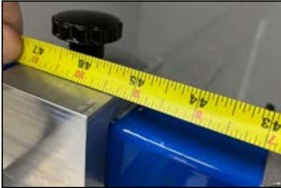
SET THE NEW BLOCK FOR THE CENTERLINE DEVICE TO 45-1/4 INCH FROM THE END OF THE REFEREE & ATTACH THE LONG CENTERLINE ANGLE TO THE BLOCK
