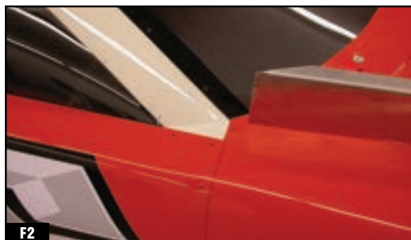
BOTH FENDER TEMPLATES ARE LOCATED AT THE INSIDE OF THE WINDSHIELD POST.
