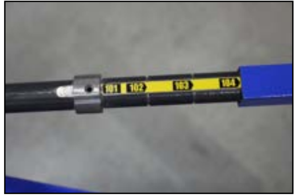
WHEELBASE IS MEASURED BY VIEWING THE CALIBRATED ARM ON THE REAR ARM.
