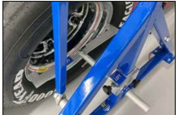
CENTER THE LEFT FRONT AS NEEDED
