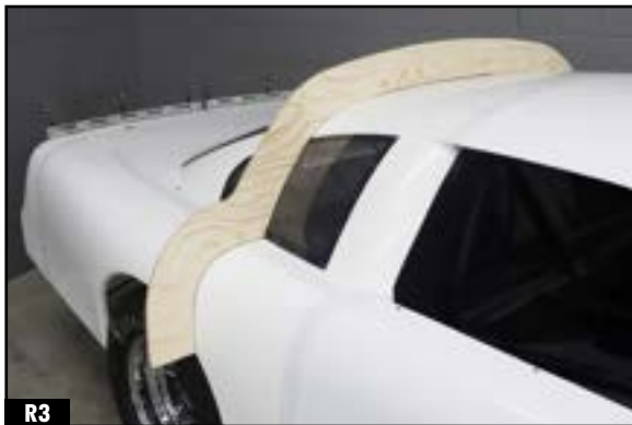
THE UPDATED AND ENHANCED SIDE-TO-SIDE TEMPLATE IS LOCATED AT THE TOP OF THE REAR WINDOW AT A 90 DEGREE ANGLE TO THE ROOF.
