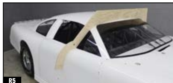
THE UPDATED AND ENHANCED SIDE-TO-SIDE TEMPLATE IS LOCATED AT THE TOP OF THE WINDSHIELD AT A 90 DEGREE ANGLE TO THE ROOF.
