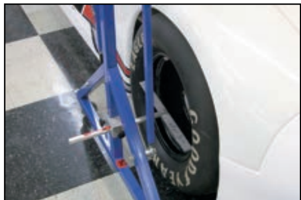
FRONT TREAD WIDTH IS MEASURED BY VIEWING GAUGE ON RIGHT SIDE MEASURING ARM.
